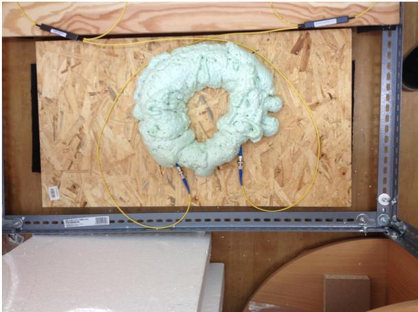
Fig. 4: Tight buffered fiber ITU-T G.652.D in mounting foam.
