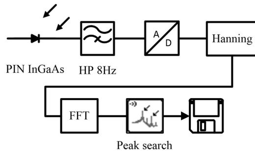
Fig. 3: Schematic diagram of electrical signal processing.
