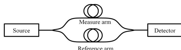
Fig. 1: Scheme of Mach-Zehnder interferometr.
