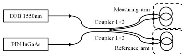
Fig. 2: Used configuration of Mach-Zehnder interferometer.
