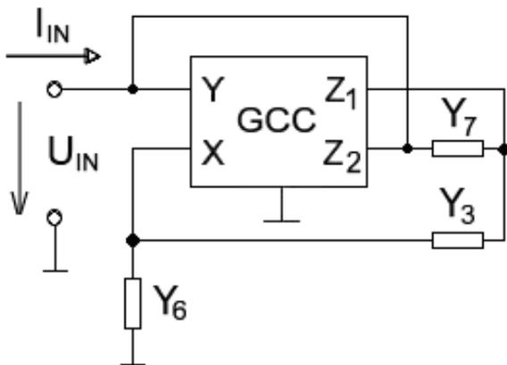
Fig. 3: General circuit structure suitable for implementation of synthetic immittance element.
