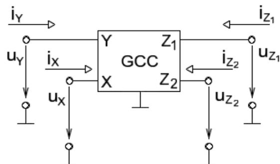
Fig. 1: Schematic symbol of four-port general current conveyor.
