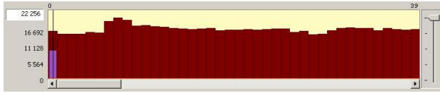
Fig. 21: The frames succession of MPEG-4 H.264/AVC compression standard with only I frames encoded to 3 Mbps by “Football” sequence.
