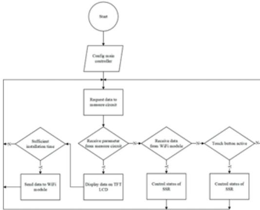
Fig. 8: Flowchart for processing data from the measuring circuit of the main control circuit.
