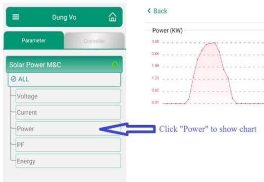
**Fig. 17:** The function to view measurement parameters and graphs on the application.
