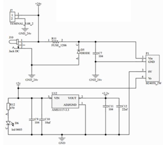
Fig. 2: Schematic diagram of the power supply block.
