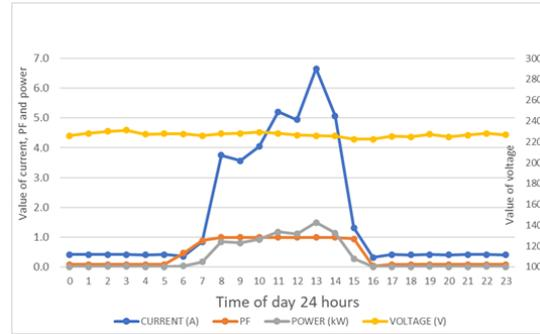
Fig. 11: Measured parameters of the solar power source during the day with the lowest generating capacity.
