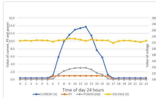
Fig. 12: Measured parameters of the solar power source during the day with the highest generating capacity.
