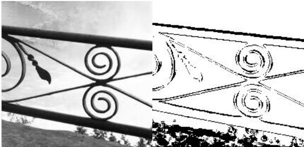
Fig. 6: Example of fuzzy image processing – edge detection, left: input image, right: output image with detected edge points.
