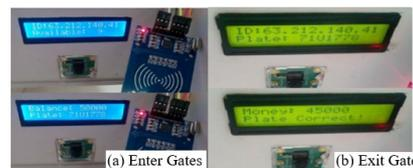
Fig. 2: RFID sensors at gates. (a) Enter gates (left). (b) Exit gates (right).
