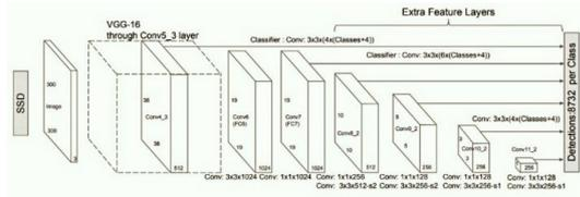
Fig. 8: SSD network architecture.
