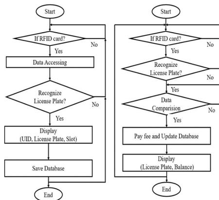
Fig. 5: (a) Entrance algorithm flowchart (left). (b) Exit algorithm flowchart (right).
