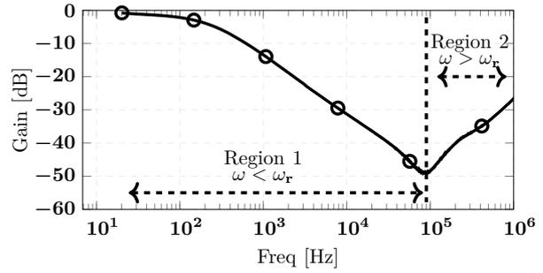
**Fig. 2:** Typical voltage gain frequency response of induction machine.
