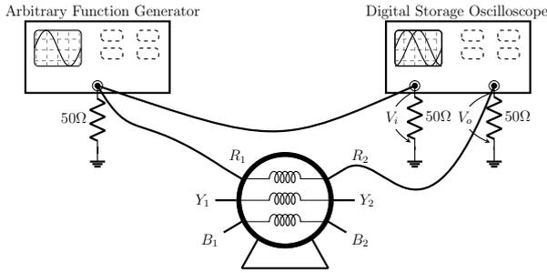
(a) Connection for winding measurement.
