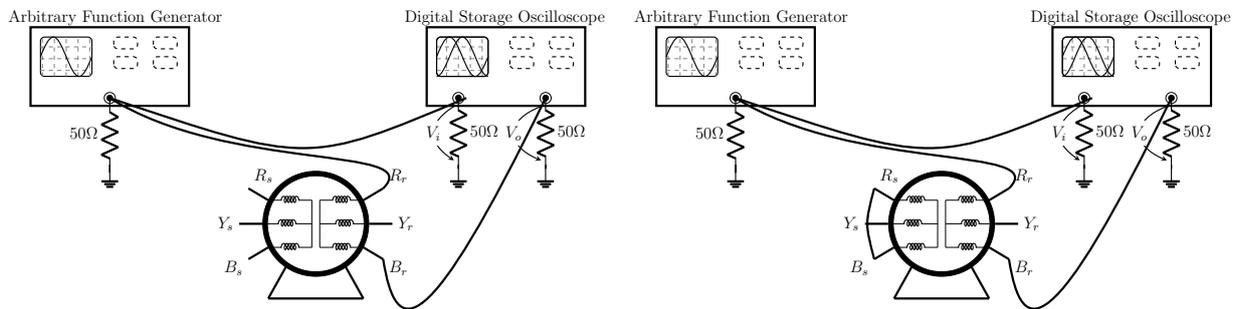
(c) Rotor winding frequency response (stator terminal open). (d) Rotor winding frequency response (stator terminal short).
