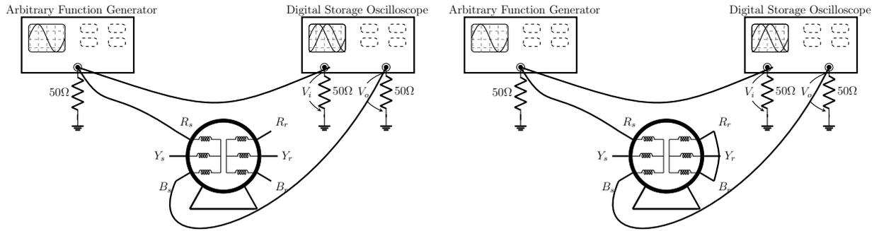
(a) Stator winding frequency response (rotor terminal open). (b) Stator winding frequency response (rotor terminal short).
