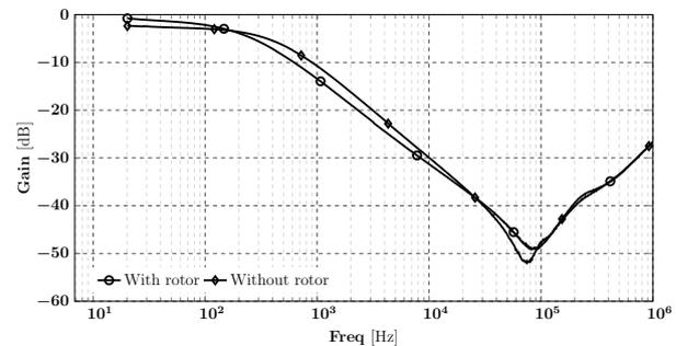
Fig. 5: Effect of core inductance on frequency response of machine 2.
