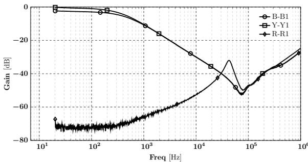
Fig. 3: Frequency response of machine 1.
