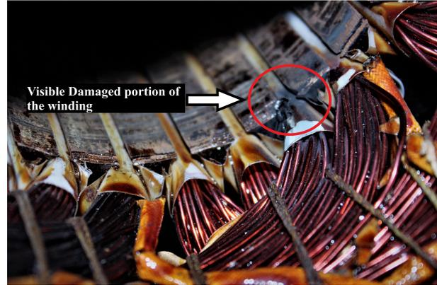
Fig. 4: Photograph of a faulty part in machine 1.
