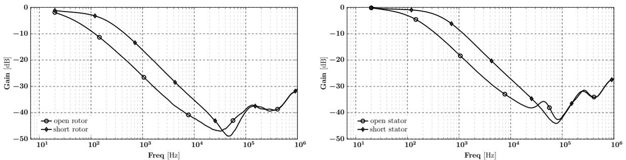
(a) Frequency response of machine 3 (stator side).
