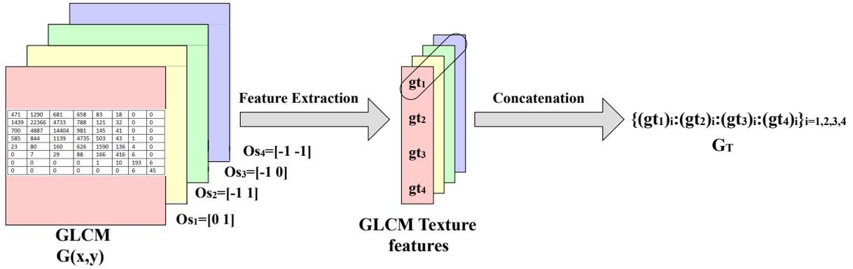
Fig. 3: Texture feature extraction from GLCM.
