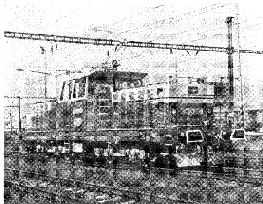
Fig. 3 The Bo'Bo', 1600 kW nominal output EL 90 E
