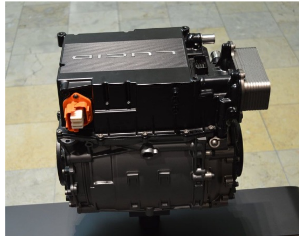
Fig. 2: Lucid air powertrain [2].
