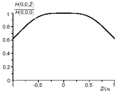
Fig. 2.: Distribution of magnetic intensity of magnetic field along the axis of Helmholtz coils
