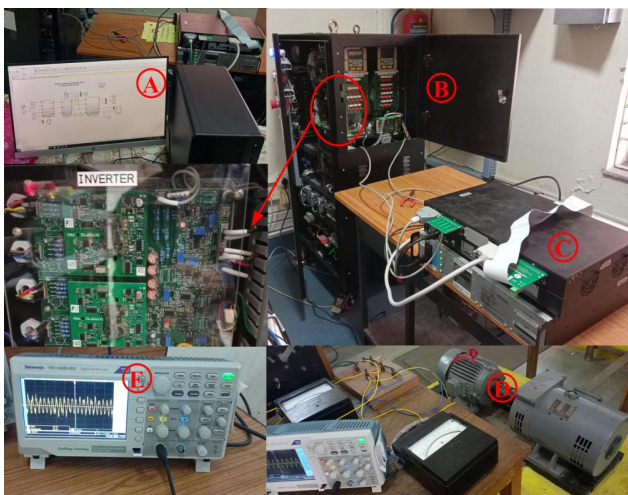
Fig. 21: Experimental setup for the proposed method. (A) Host PC, (B) 3-Phase VSI, (C) OpalRt-4510 controller, (D) Induction Motor coupled with DC generator, (E) DSO.
