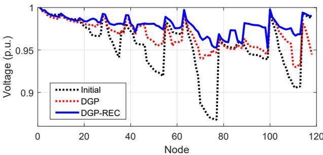
Fig. 5: The voltage profile in the 119-node DS obtained by AEO.
