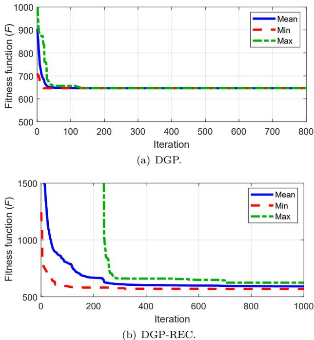
**Fig. 7:** The maximum, minimum and mean convergence curves of AEO for the 119-node DS.
