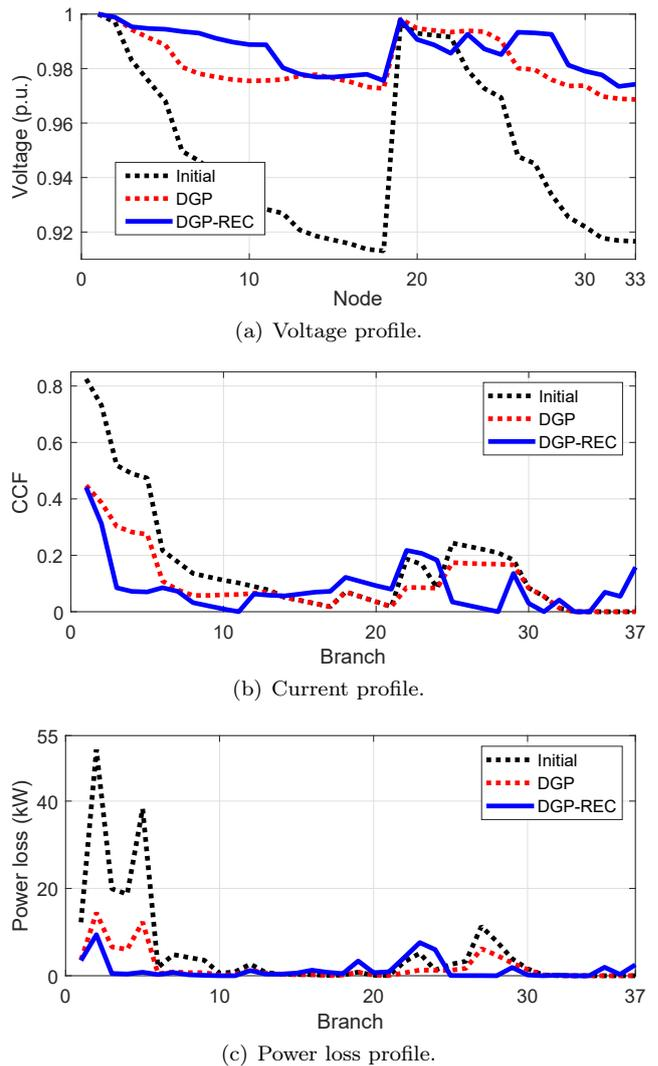
Fig. 2: The voltage (a), current (b) and power loss (c) profiles in the 33-node DS obtained by AEO.
