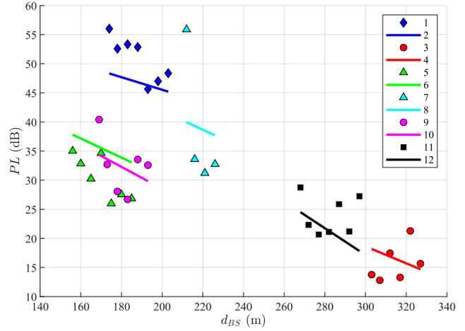
**Fig. 6:**  $\xi(x)$  variation behind the buildings and comparisons with the straight-line approximation results for the UMTS technology: 6 m experiment - 1, 14 m experiment - 3, 18/1 m experiment - 5, 18/2 m experiment - 7, 23 m experiment - 9, 32 m experiment - 11, 6 m model - 2, 14 m model - 4, 18/1 m model - 6, 18/2 m model - 8, 23 m model - 10, 32 m model - 12.
