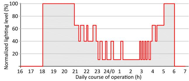
Fig. 1: Example of a quadri-power detector-driven operational profile.
