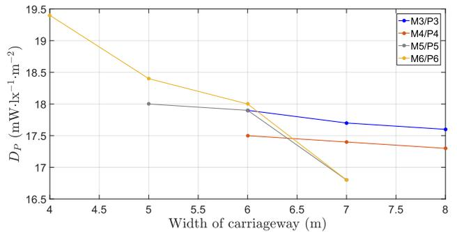
Fig. 8: Typical values of the Power Density Indicator  $D_P$  in  $mW \cdot lx^{-1} \cdot m^{-2}$  for road profile D.
