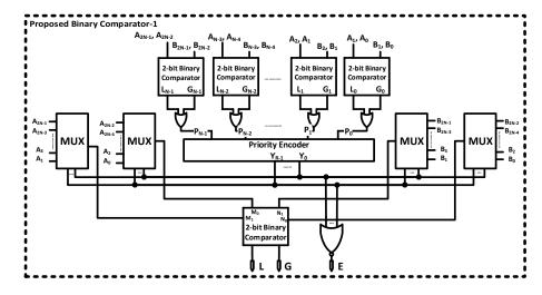
Fig. 2: Proposed architecture-1 for 2N-bit binary comparator system using a 2-bit elementary binary comparator.
