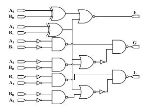
Fig. 1: Gate level schematics of 2-bit binary comparator [33].
