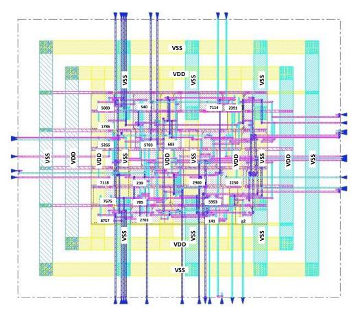
Fig. 8: The physical layout of the proposed 16-bit binary comparator using a 4-bit elementary comparator.
