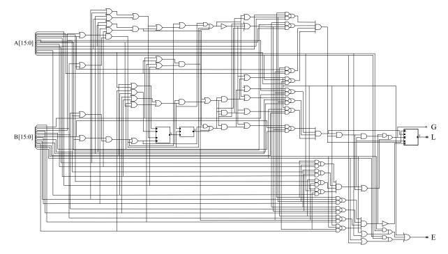
Fig. 5: RTL schematics of proposed 16-bit binary comparator using a 2-bit elementary comparator.
