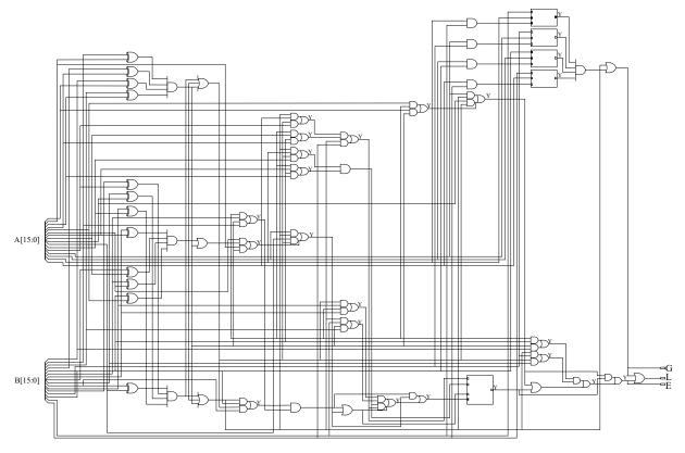
Fig. 6: RTL schematics of proposed 16-bit binary comparator using a 4-bit elementary comparator.
