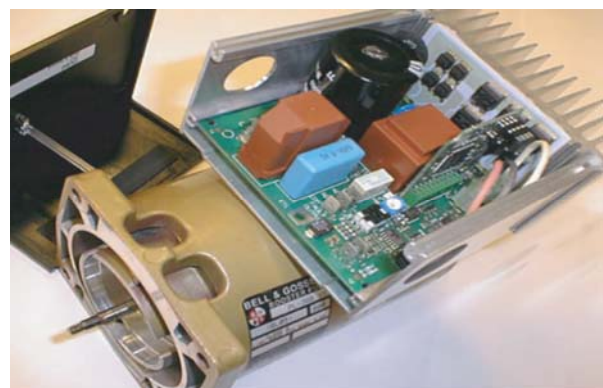
Fig. 1: Two-phase drive using voltage inverter and 3-phase low-cost motor [4].
