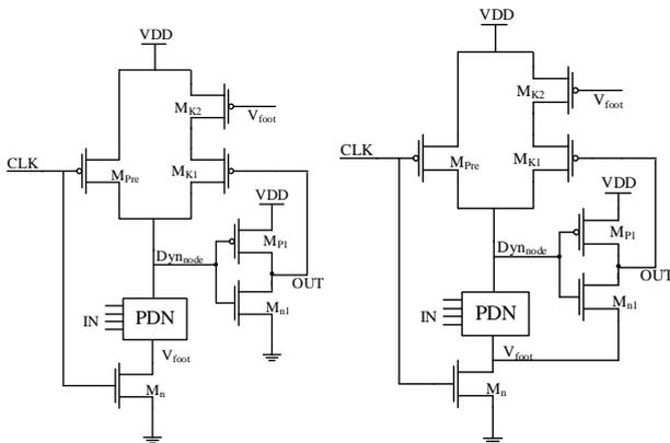
(a) Footer Voltage Controlled Dual Keeper (FVCDK). (b) Footer Voltage Controlled Dual Keeper with Static Switching (FVCDK-SS).
