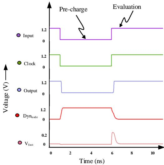
Fig. 7: Output waveform of the proposed circuit during pre-charge and evaluation phase.
