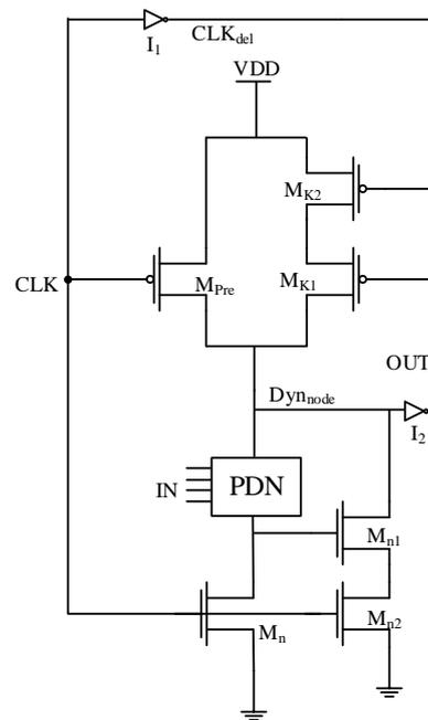
Fig. 4: Clock Delayed Dual Keeper with Additional Discharge Path (CDDK-ADP) [10].
