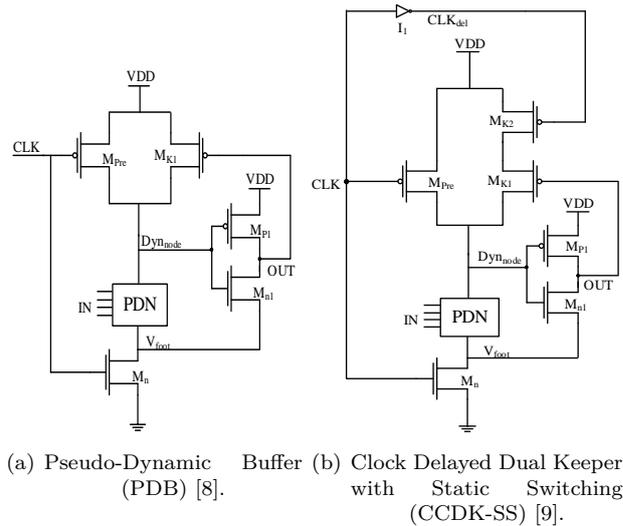
Fig. 3: Domino Logic with Static Switching.
