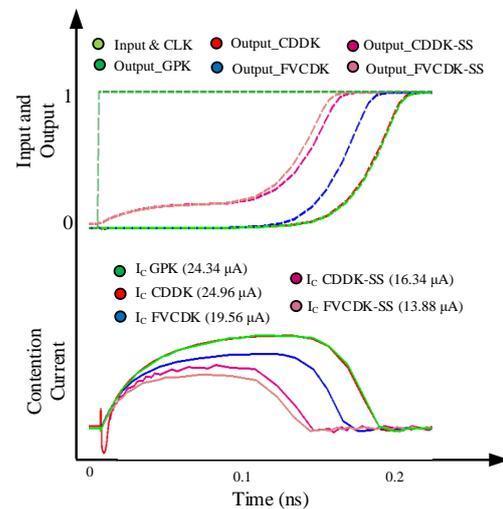
Fig. 10: Contention current obtained for GPK, CDDK, CDDK-SS, FVCDK and FVCDK-SS.
