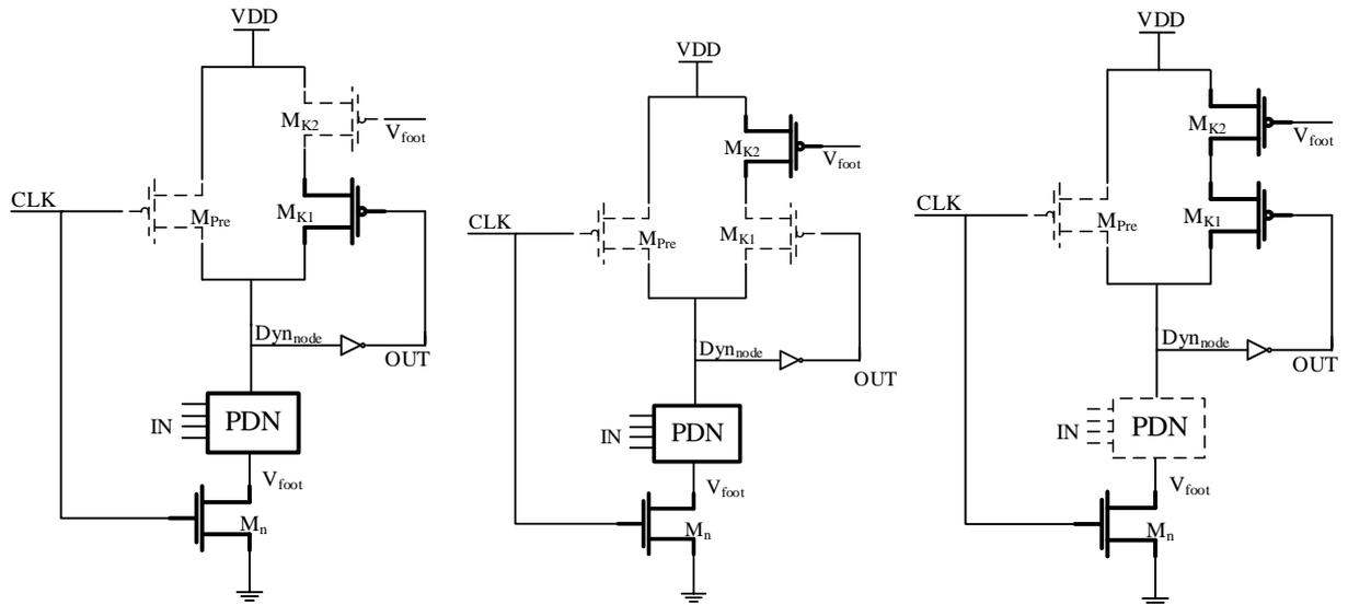
(a) During initial evaluation phase if PDN is TRUE. (b) During evaluation phase if PDN is TRUE. (c) During evaluation phase if PDN is FALSE.
