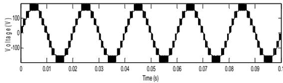
Fig. 17: Pole voltage  $f_c = 4$  kHz.
