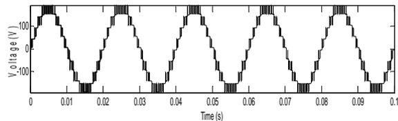
Fig. 11: Pole voltage  $f_c = 2$  kHz.
