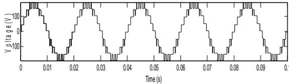
Fig. 8: Pole voltage  $f_c = 1$  kHz.
