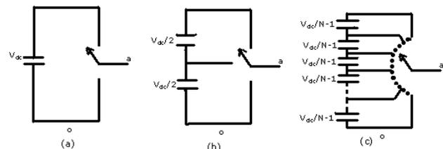
**Fig. 1:** Schematic Diagram of (a) Two level inverter (b) Three level inverter (c) N level inverter.
