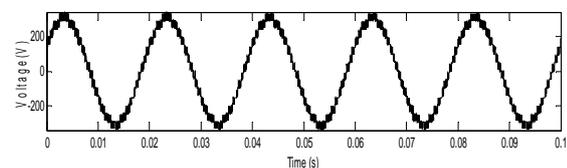
Fig. 19: Line voltage  $f_c = 4$  kHz.
