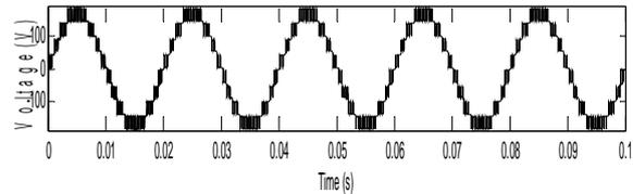
Fig. 14: Pole voltage  $f_c = 3$  kHz.
