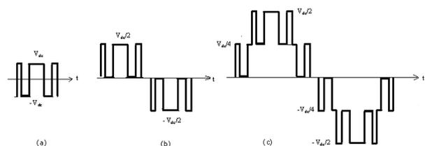
**Fig. 2:** Output voltage of (a) Two level inverter (b) Three level inverter (c) Five level inverter.
