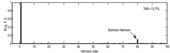
Fig. 7: Pole voltage THD  $m_f = 80, f_c = 4$  kHz.
