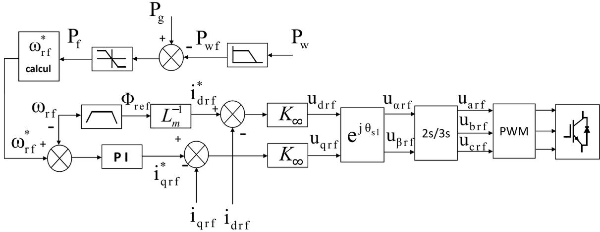
Fig. 3: Control Structure of the rotor side converter with  $H_\infty$  controllers.
