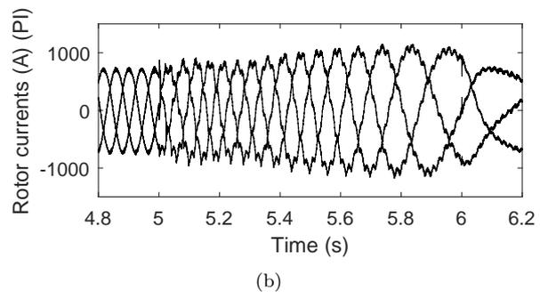
Fig. 12: Influence of dip voltage on PI controller (a) WRIM rotor currents (b) Zoom of the rotor currents.
