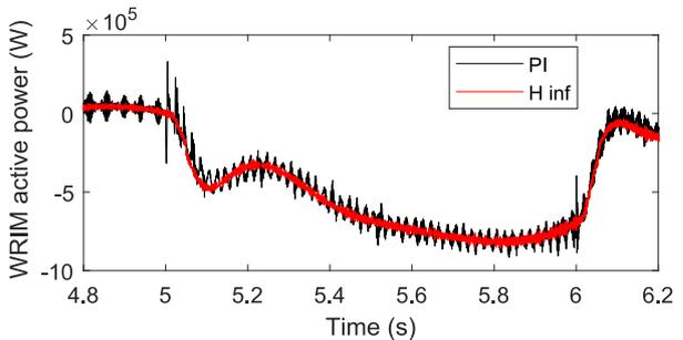
**Fig. 17:** Zoom of WRIM active power under voltage dip with parameter perturbation.
