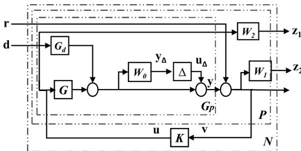
Fig. 5: The  $H_\infty$  controller design.
