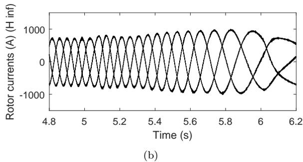
Fig. 13: Influence of voltage dip on  $H_\infty$  controller (a) WRIM rotor currents (b) Zoom of the WRIM rotor currents.
