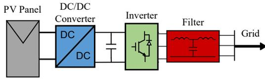
Fig. 1: The structure of a grid-connected PV panel.
