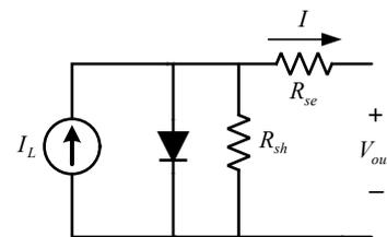
Fig. 3: One-diode model of a PV cell.
