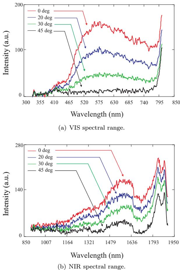
**Fig. 2:** Spectra of light transmitted through the polariscope with inserted sample of PMMA for various angles of rotation obtained in VIS and NIR spectral ranges.
