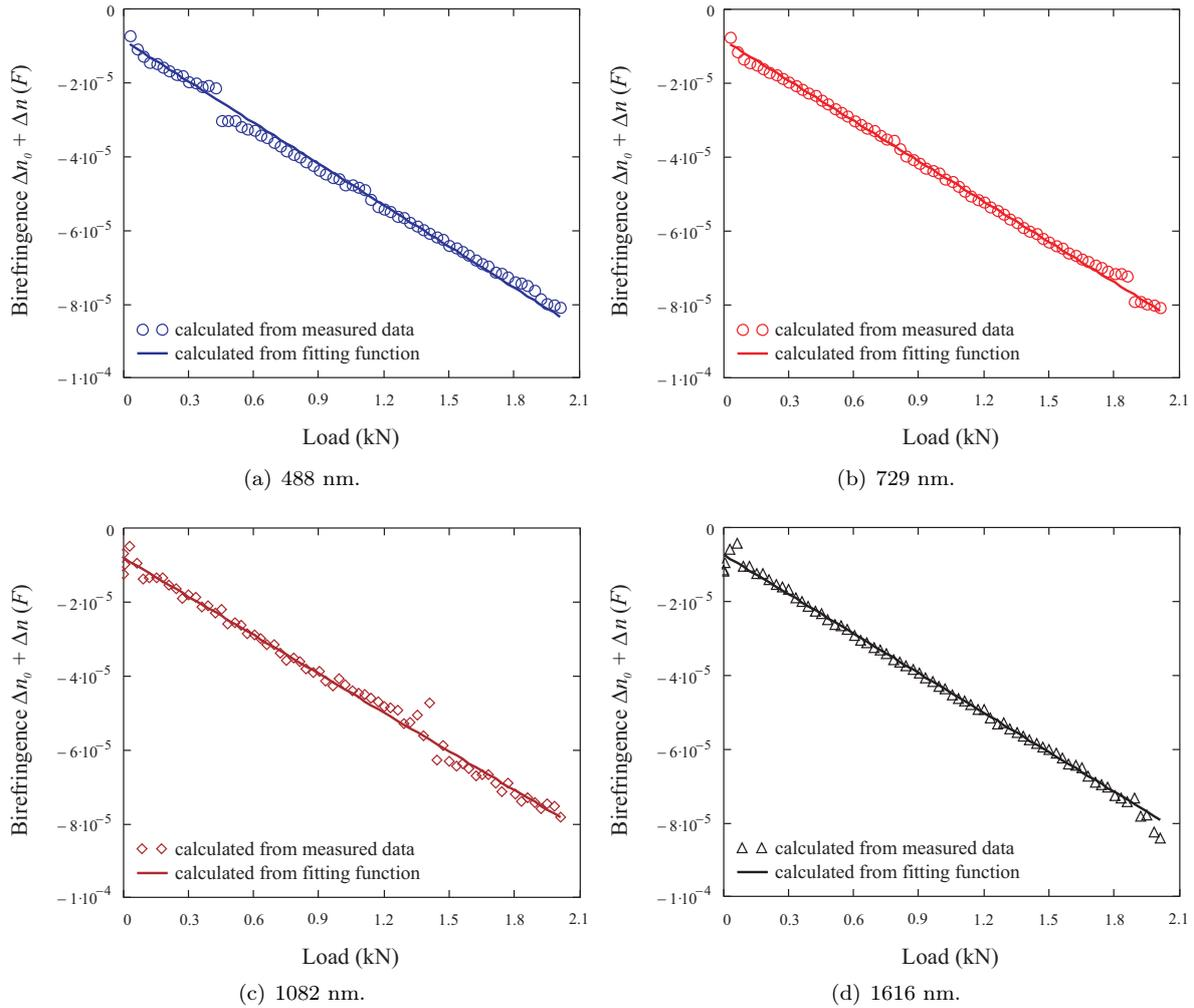
**Fig. 7:** Total birefringence as function of the load plotted for wavelengths 488 nm, 729 nm, 1082 nm and 1616 nm.
