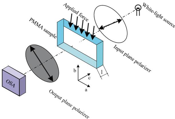
**Fig. 1:** Apparatus for investigation of birefringence of a medium. Arrows drawn inside the polarizers show the orientation of the planes of polarization. OSA - Optical Spectrum Analyzer.
