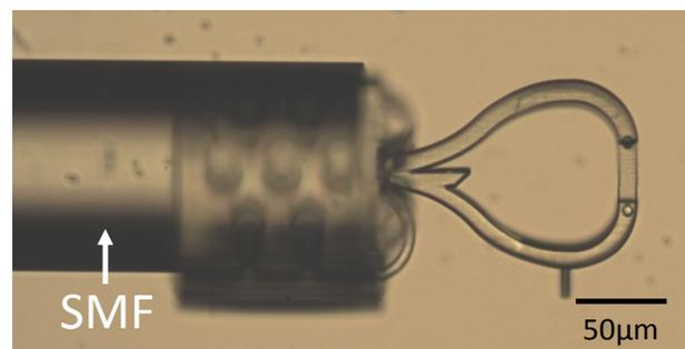
**Fig. 4:** Optical microscope image of final connection of the Single Mode optical Fiber (SMF) with prepared structures separated from the substrate.
