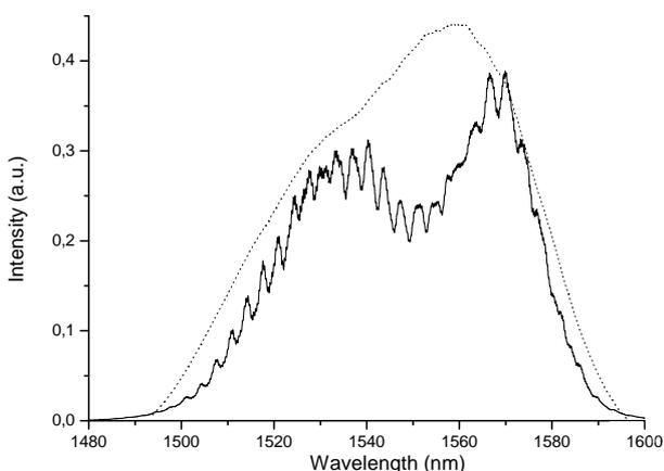
**Fig. 7:** Transmission spectral characteristic of the prepared Mach-Zehnder interferometer device and reference spectrum of the used light source (dotted line).
