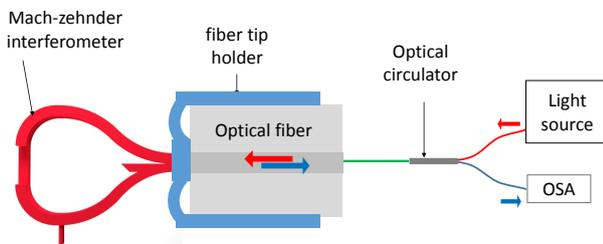
**Fig. 6:** Measurement setup for optical characterization of the prepared devices on fiber tip.
