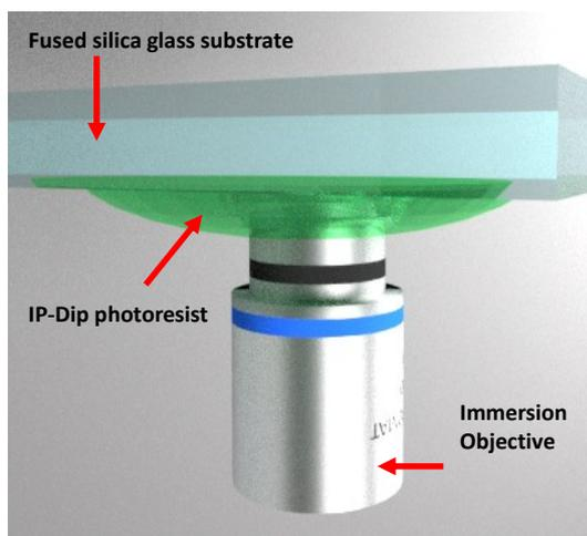
**Fig. 1:** DiLL configuration, the liquid Dip photoresist is dropped on substrate and turned upside down, objective is immersed in photoresist during DLW process [6].
