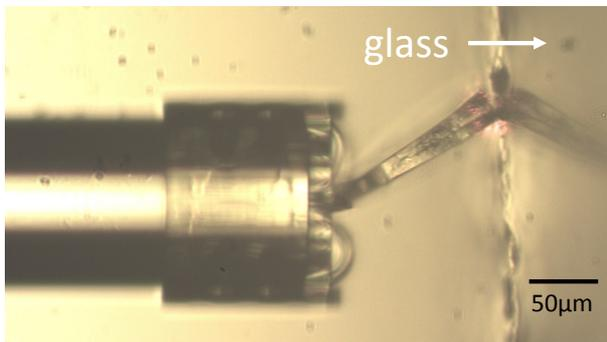
**Fig. 5:** Optical microscope image of depressed structure applied on the optical fiber.
