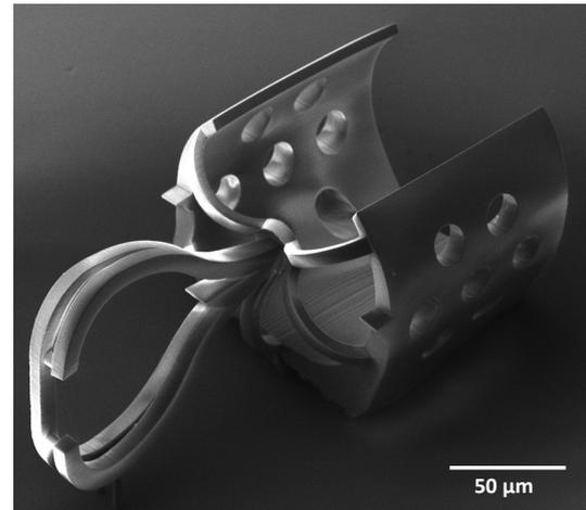
**Fig. 3:** SEM image of the prepared 3D MZI-based structure on fused silica substrate.
