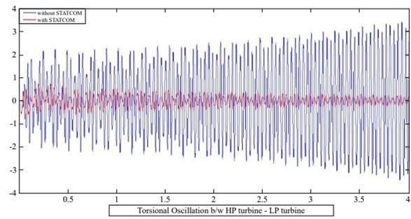
Fig. 7: Variation in torque between HP-LP turbine with use of static synchronous compensator.
