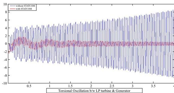
Fig. 6: Variation in torque between IP turbine and generator with application of static synchronous compensator.
