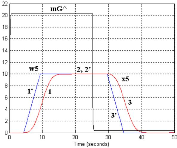
Fig.11 Reference  $w_5 [m]$  and real  $x_5 [m]$  crane crab position
