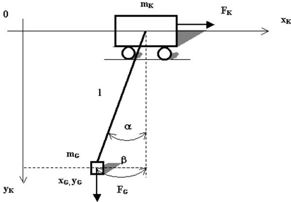
Fig.2 Mechanical part of the crane crab and bridge
