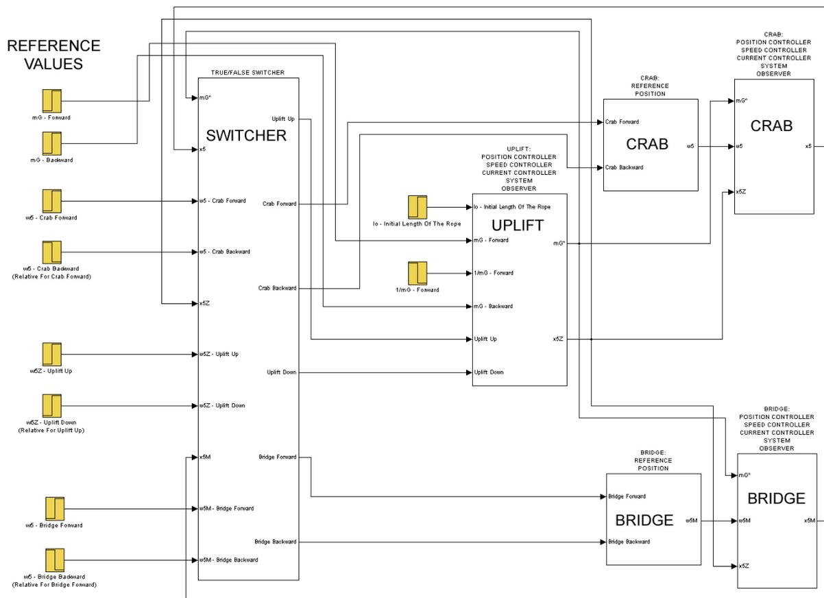
Fig.9 Simulation scheme of crane from MATLAB Simulink
