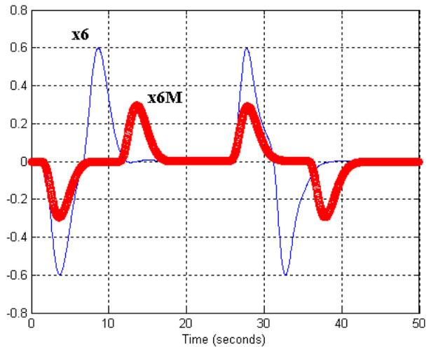
Fig.14 Burden deviation at crane crab  $x_6 [m]$  and bridge  $x_{6M} [m]$  motion
