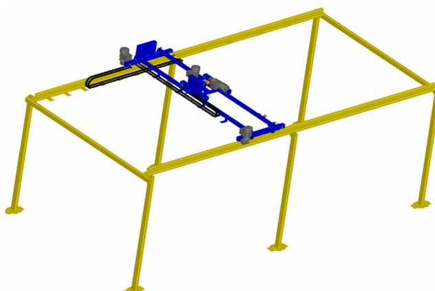
Fig.1 Model of double cross-beam bridge crane
