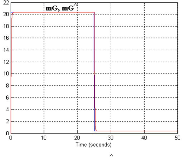
Fig.13 Real  $m_G [t]$  and observed  $m_G [t]$  burden weight
