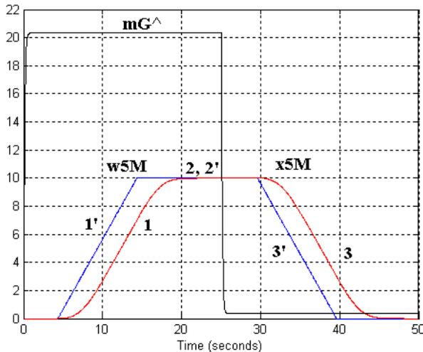
Fig.12 Reference  $w_{5M} [m]$  and real  $x_{5M} [m]$  crane bridge position
