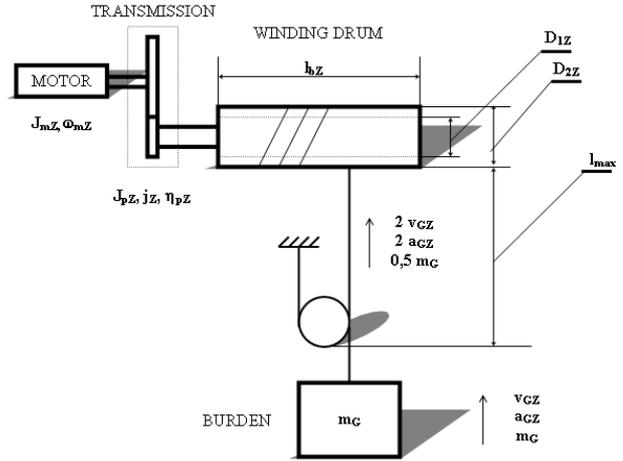
Fig.3 Mechanical part of the crane uplift
