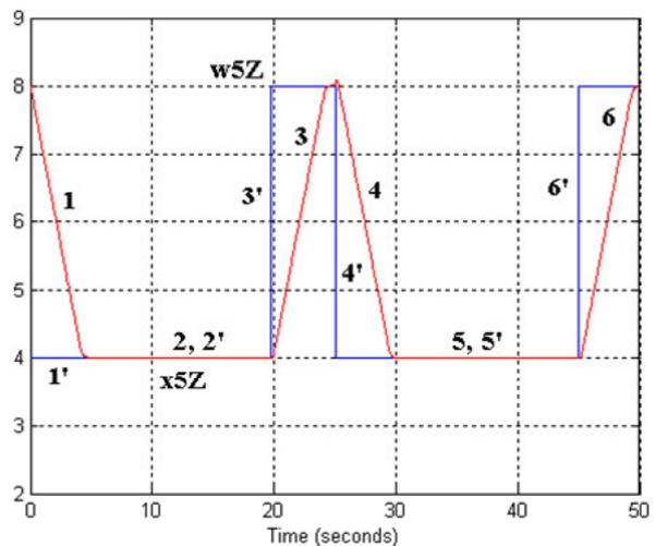
Fig.10 Reference  $w_{5Z}$  [m] and real  $x_{5Z}$  [m] crane uplift at burden transport
