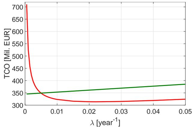
**Fig. 2:** Dependency of the cost on failure intensity (failures per year) - TCO without the intended price increase at lower failure rate (green line), total TCO (red line).
