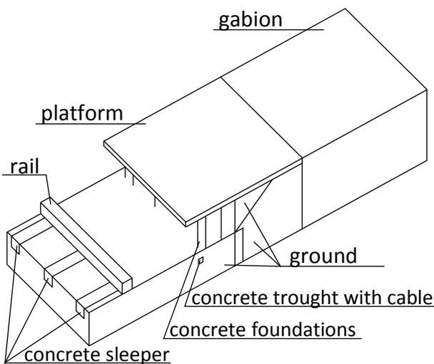
Fig. 1: Geometric layout of the model.
