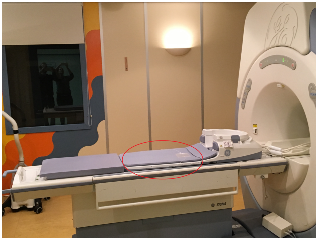
Fig. 4: A photo of the sensor pad positioned within the MRI Scanner's bed (encircled with red color).
