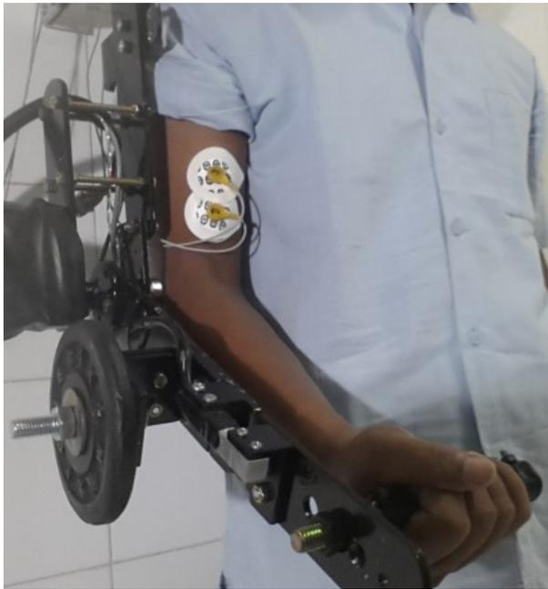
**Fig. 1:** The exoskeleton frame to synchronize the elbow joint motion (flexion and extension).
