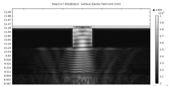
Fig. 10: Electric field distribution in structure for designed finger length and distance between ohmic contacts as depicted.
