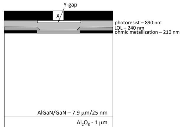
**Fig. 2:** The structure used for simulations in COMSOL.
