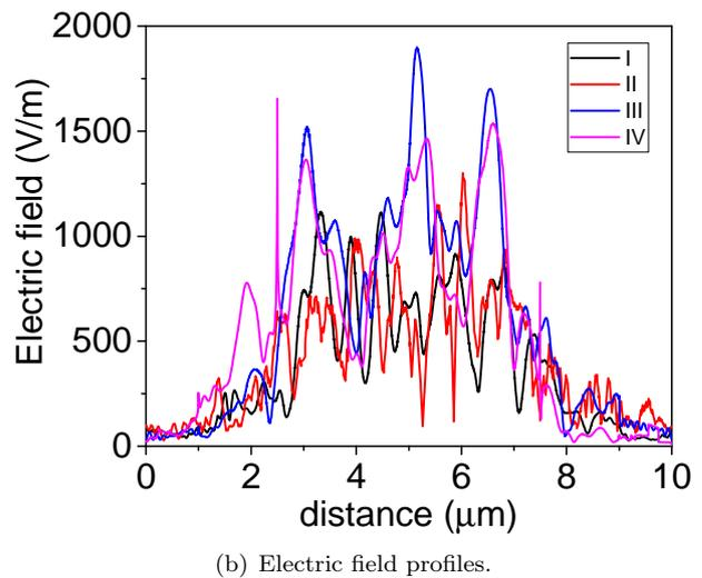
Fig. 11: Electric field distribution and profiles in structure for designed finger length and distance between ohmic contacts of 5  $\mu\text{m}$  and 8  $\mu\text{m}$ .
