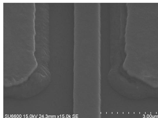
**Fig. 5:** SEM image of test structure finger between ohmic contacts paths.
