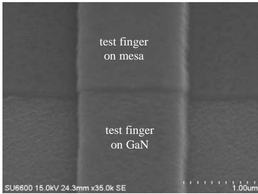
Fig. 6: SEM image of test structure finger on various areas.
