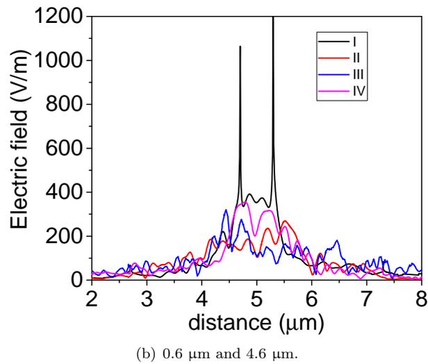
Fig. 9: Electric field profiles in structure for designed finger length and distance between ohmic contacts as depicted.
