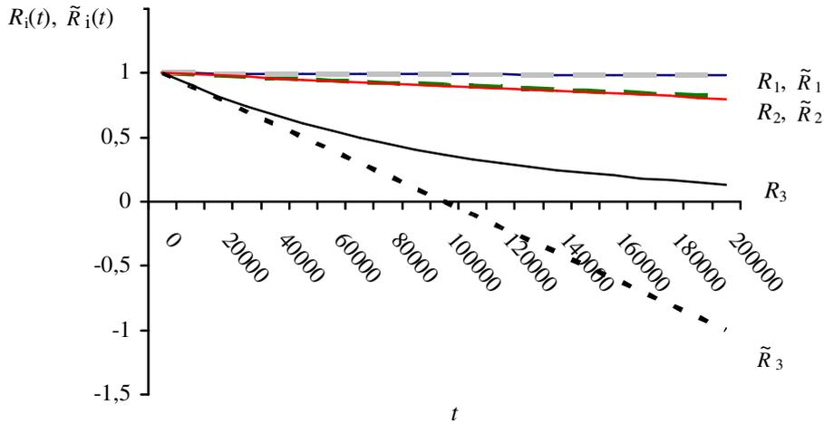
Fig. 3. The comparison between element reliable operation probabilities values calculated by equations for exponential distribution and exponential distribution approximation.
