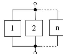
Fig. 2. The parallel system block diagram.
