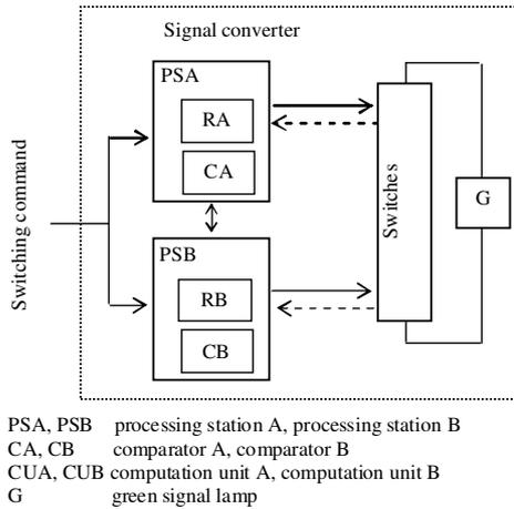
Fig. 5. The block diagram of the signal converter for green railway signal control.
