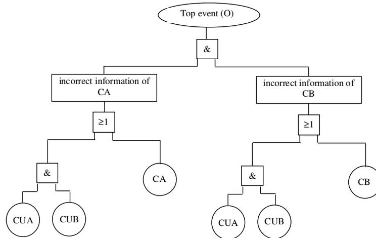
Fig. 6. The failure state tree for system failure state occurrence analysis.
