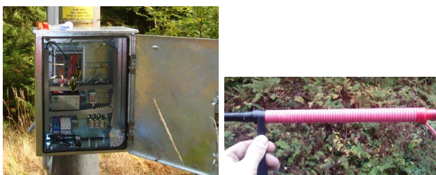
Fig. 10: Fault detector and a detail of a sensor (a single layer coil with 75 turns).
