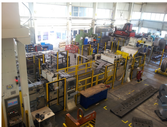
Fig. 7: Belt feeder of sheet steel for the forging press.
