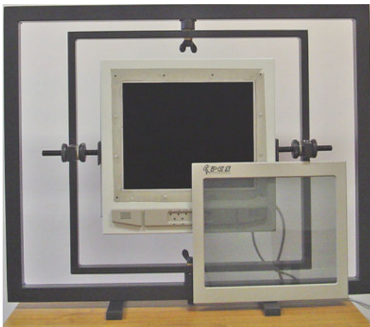
Fig. 2 Measured LCD display steady in the mechanical support.
