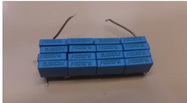
Fig. 12: View of the series-parallel connection of capacitors - 33 nF.
