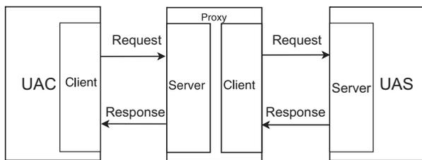
Fig. 3: Communication between SIP devices.
