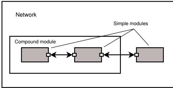
Fig. 1: Simple and compound modules.
