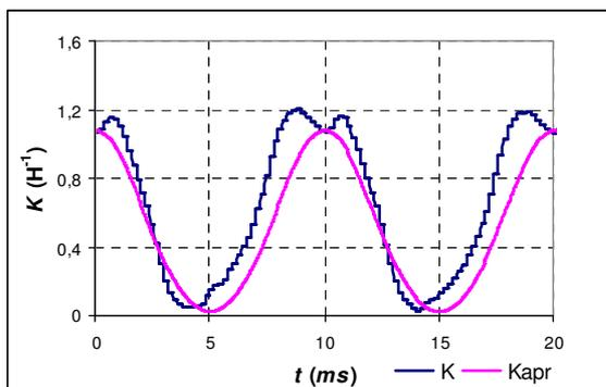
Fig. 4 The instantaneous inverse inductance  $K_k(t_i)$
