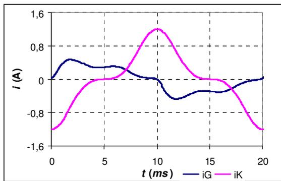
Fig. 6. The current waveform  $i_{Cpr}(t_i)$  and  $i_{Kpr}(t_i)$
