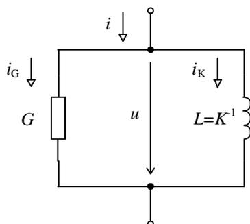
Fig. 1. The linear model of the transformer cross section
