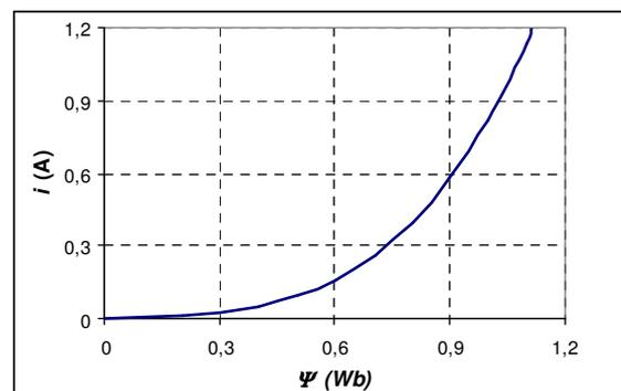
Fig. 5. The magnetization characteristic
