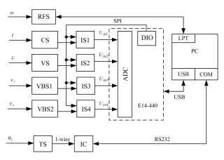
Fig. 4: Structure of the measuring complex.
