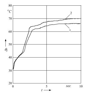
Fig. 5: Results of the change of the EM winding slot temperature: 1 – undamaged EM; 2 – EM with a damage.
