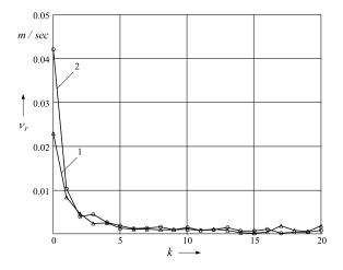
Fig. 6: Results of spectral analysis of a radial component of vibration: 1 – undamaged EM; 2 – EM with a damage.
