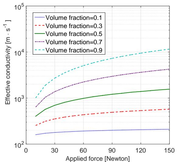
Fig. 6: Effective conductivity of SiO<sub>2</sub>/Epoxy composites.
