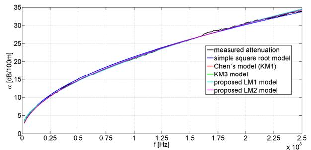
Fig. 1: Measured and modeled attenuation constants for UTP cat. 5.
