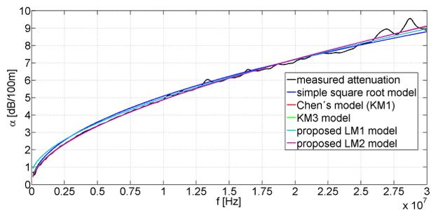
Fig. 13: Attenuation constants for TCEKFLES cable.
