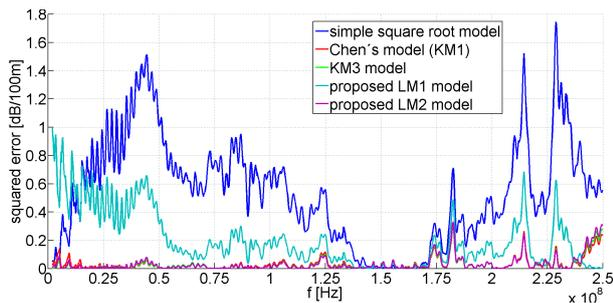
Fig. 4: Squared error characteristic for each model for UTP cat. 6.
