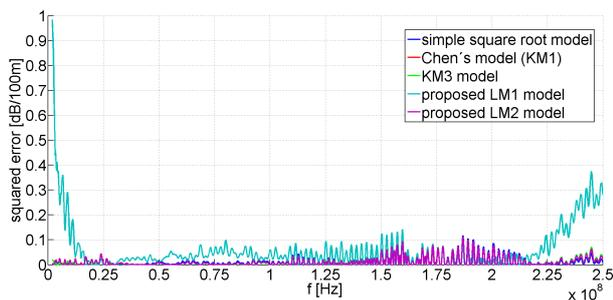
Fig. 6: Squared error characteristic for each model for STP cat. 7.
