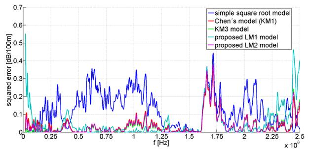
Fig. 2: Squared error characteristic for each model for UTP cat. 5.
