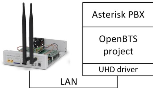
Fig. 3: USRP N210 connected with host OpenBTS server.
