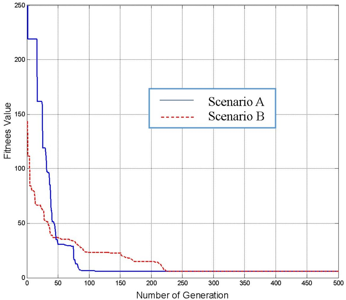
Fig. 4: Convergence characteristic for PSO-TVAC.
