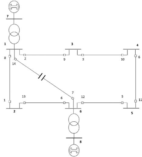
Fig. 3: Single line diagram of 8-bus system.
