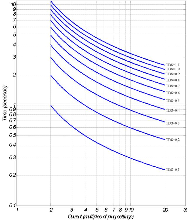
Fig. 1: Typical time/current characteristics of standard IDMT relay.
