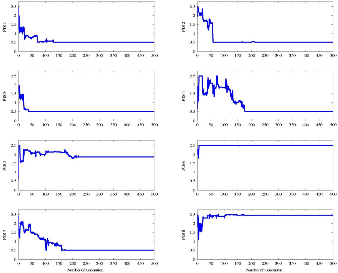
Fig. 7: Convergence evolution of control variable PTS associated to relays 1-8 during search process.
