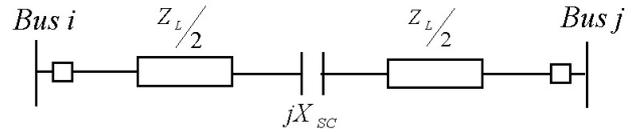
Fig. 2: The single line of a simplified series compensated system.
