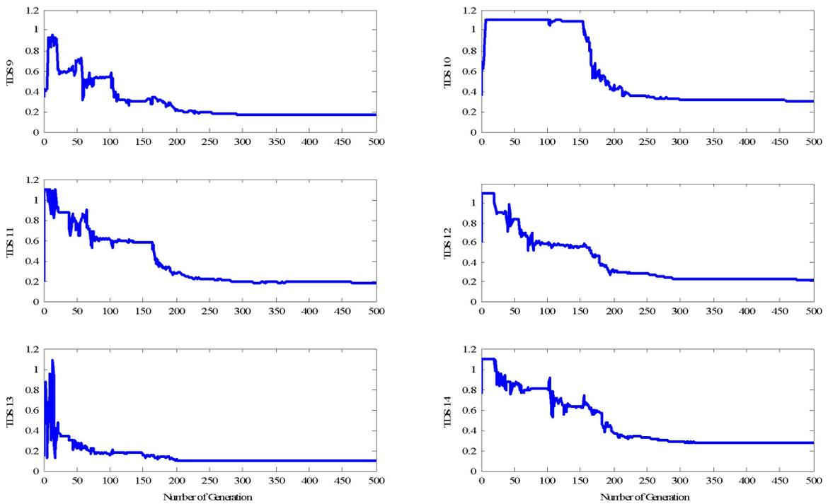
Fig. 6: Convergence evolution of control variable TDS associated to relays 9-14 during search process.
